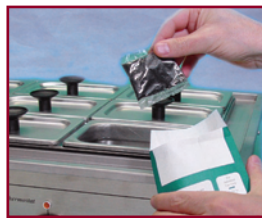
Drop dye packet into dye tank (vat) filled with water. Plastic and ingredients dissolve in water.
