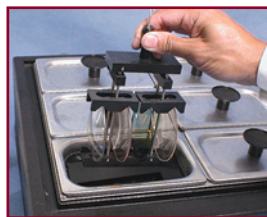
Dye heating unit is needed to heat dye solutions. Lenses are dipped in hot dye bath at 200 - 205°F (93.3 - 96.1°C) by using a lens holder.
