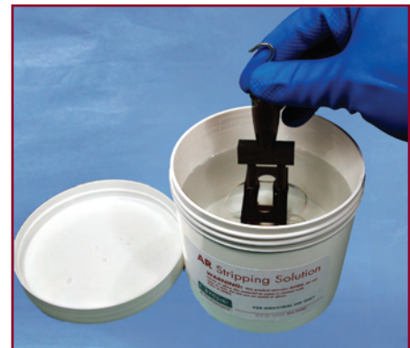
Lenses are dipped into the AR Solution for 30 seconds to 3 minutes, then rinsed with water
