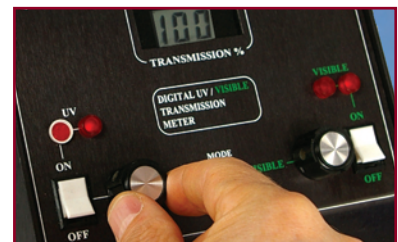
Calibrate to 100% UV or visible light transmission
