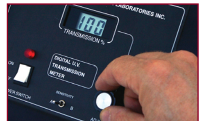
Calibrate to 100% UV light transmission Flip switch from A to B to extend bulb life.
