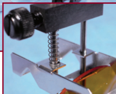
Certain models offer spring loaded locks to prevent slippage while tinting.
